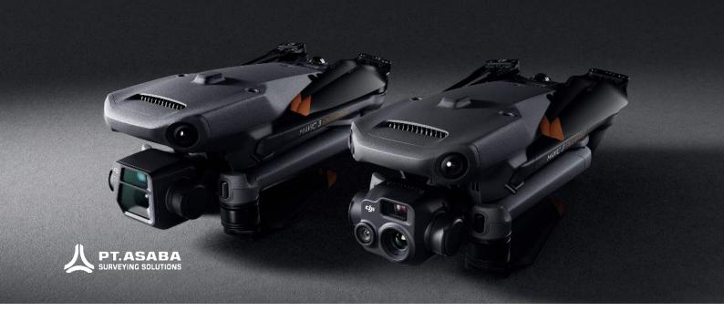
The Mavic 3 Enterprise redefines industry standards for small commercial drones. With a mechanical shutter, a 56× zoom camera, and an RTK module for centimeter-level precision, the Mavic 3E brings mission efficiency to new heights. A thermal version is available for firefighting, search and rescue, inspection, and night operations.
